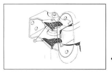
DOOR JAMB SWITCH 1062F, 1062DF, 1063F, 1064DF, 1263F, 1271, 2271 2263F, 2562, 2562DF, 2563F, 2564DF Apply light coat of #630 AA Lubriplate or its equivalent.
