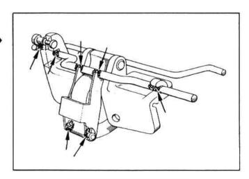
LIFT GATE HINGE ASSEMBLY 1062F, 1062DF, 1063F, 1263F, 2263F 2562, 2562DF, 2563F
