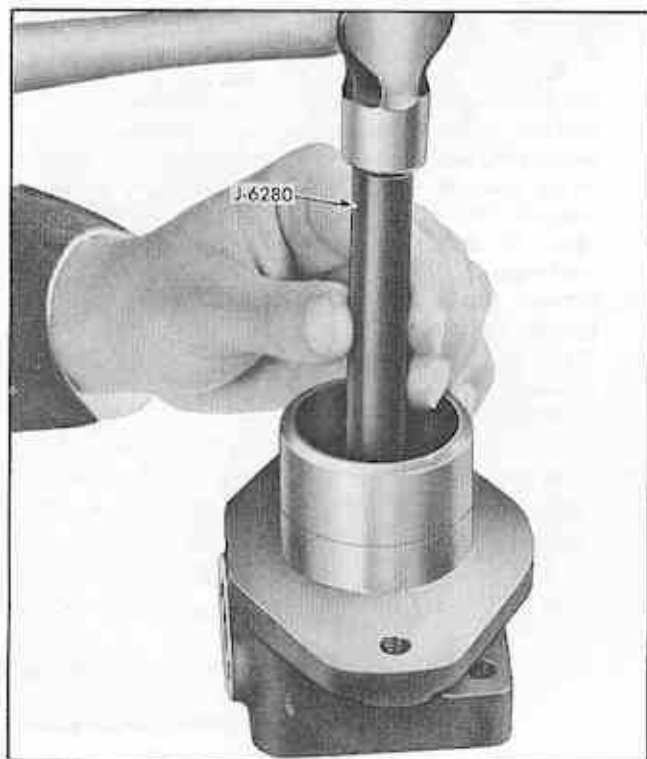
Fig. 106 Driving Needle Bearing Into Pump Body
