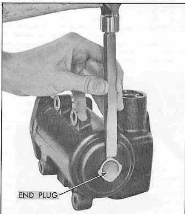
Fig. 48 Removing Housing End Plug Staked Portions
