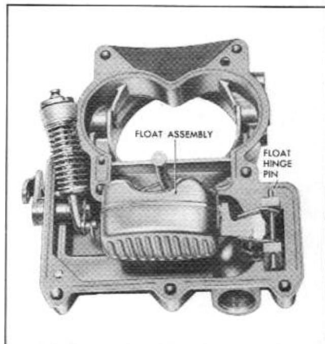
Fig. 6B-59 Float to Bowl Cover Construction
