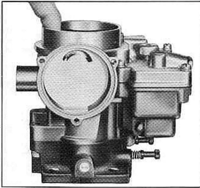
Fig. 6B-72 Replacing Choke Baffle Plate
