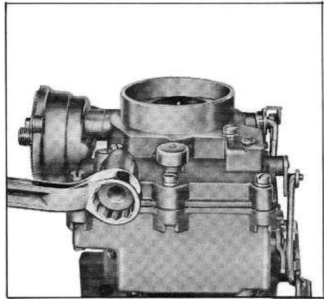
Fig. 6B-53 Removing or Replacing Filter Screen Retainer Nut
