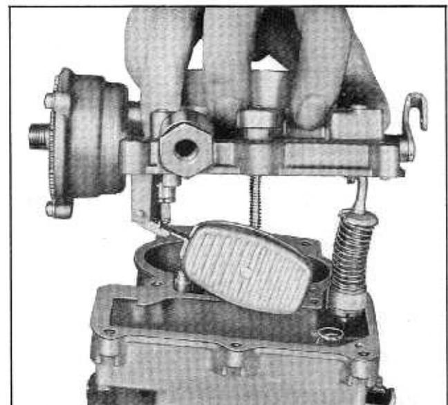
Fig. 6B-54 Removing or Replacing Bowl Cover
