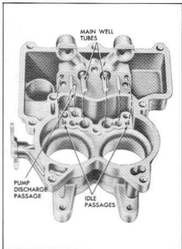
Fig. 6B-41 Passage Identification—Bowl to Cluster Assembly
