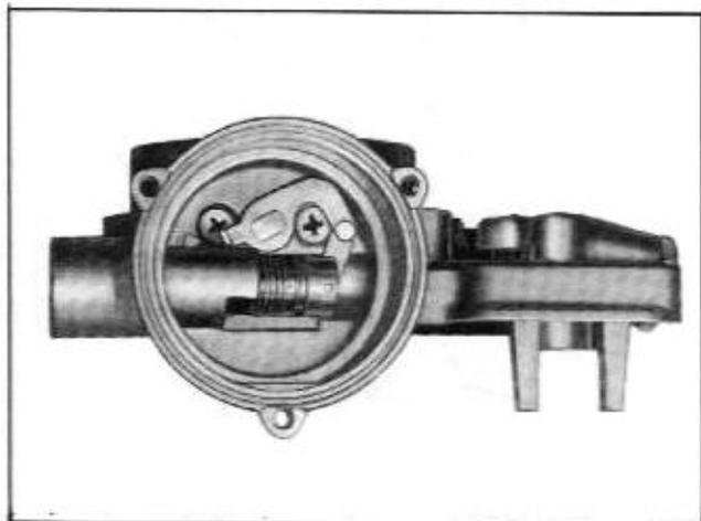
Fig. 6B-56 Removing or Replacing Choke Piston
