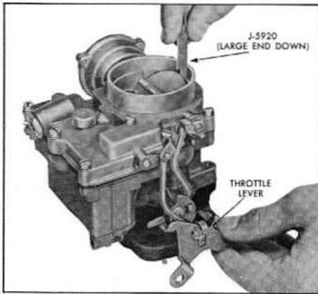
Fig. 6B-48 Checking Unloader Adjustment
