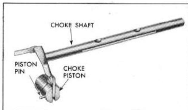
Fig. 6B-57 Choke Shaft and Piston Assembly
