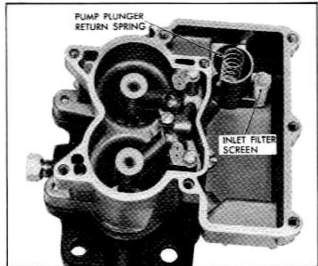
Fig. 6B-62 Pump Plunger Return Spring and Inlet Filter Screen
