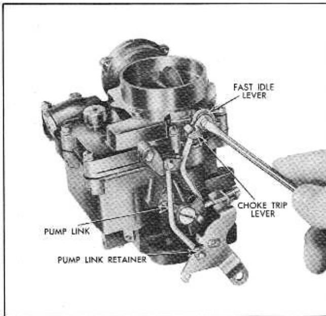
Fig. 6B-51 Removing or Replacing Choke Trip Lever
