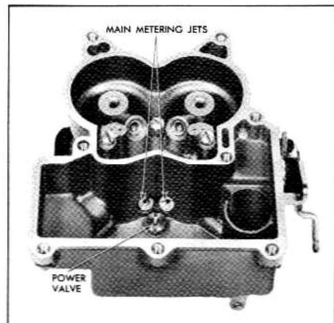
Fig. 6B-63 Main Metering Jets and Power Valve
