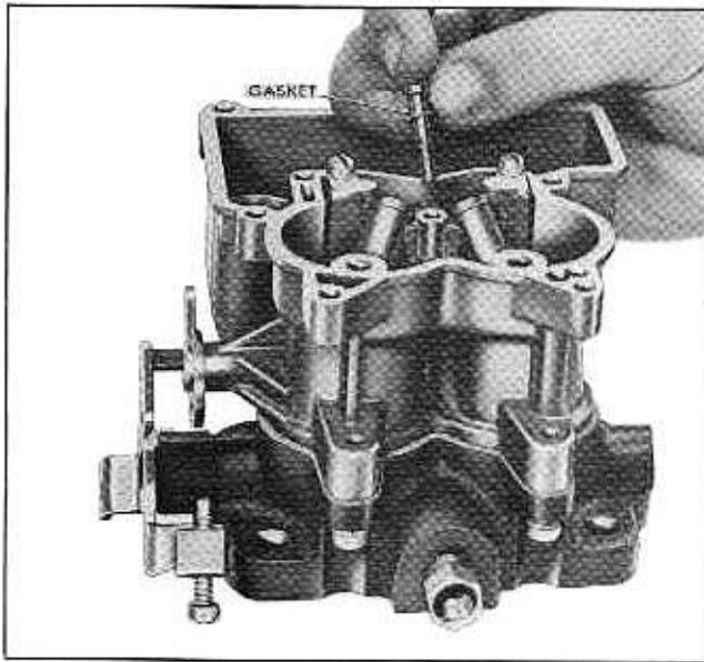
Fig. 6B-64 Removing or Replacing Cluster Assembly
