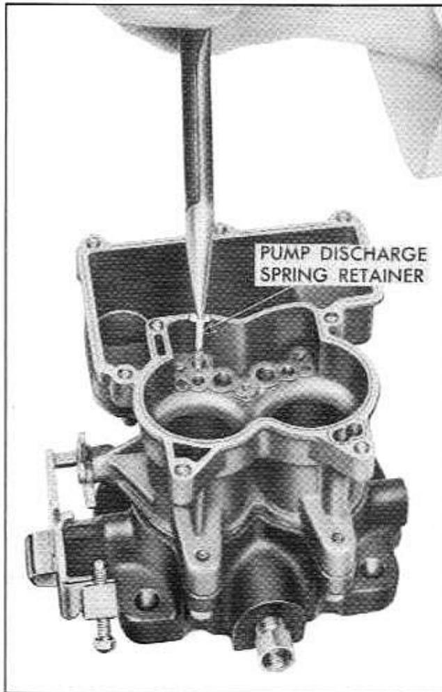
Fig. 6B-65 Removing or Replacing Pump Discharge Spring Retainer
