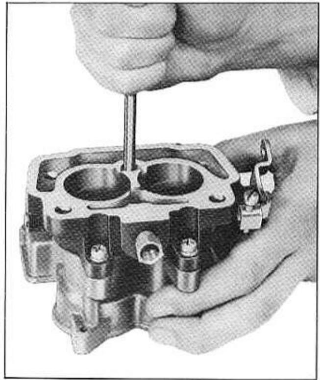
Fig. 6B-66 Removing or Replacing Throttle Body
