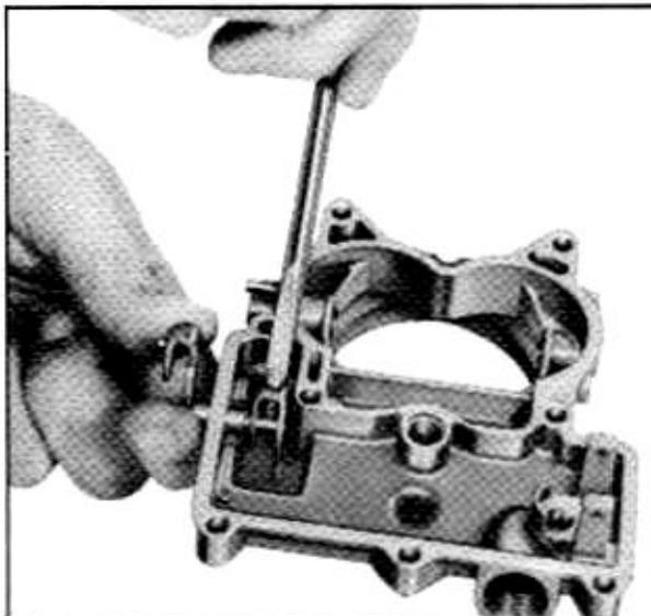
Fig. 6B-61 Removing or Replacing Pump Lever
