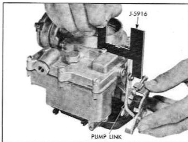
Fig. 6B-71 Checking Pump Link
