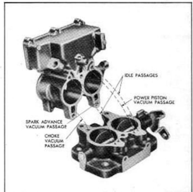
Fig. 6B-39 Passage Identification—Throttle Body to Bowl
