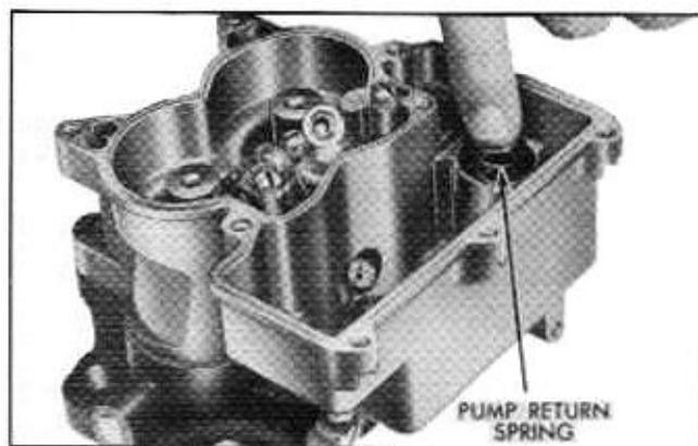
Fig. 6B-68 Replacing Pump Return Spring
