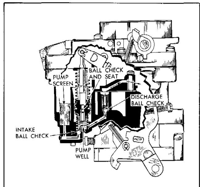
Fig. 6B-46 Accelerator Pump System
