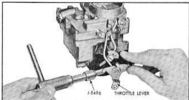
Fig. 6B-49 Adjusting Unloader with J-5496
