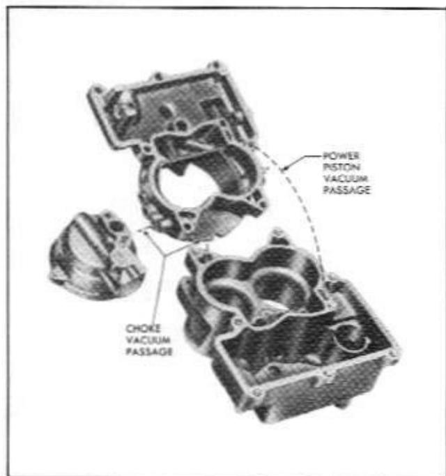
Fig. 6B-40 Passage Identification—Bowl to Cover to Choke Housing
