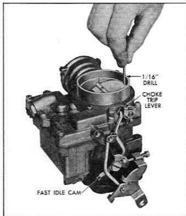
Fig. 6B-47 Checking Fast Idle Adjustment
