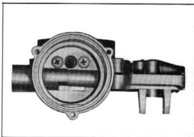
Fig. 6B-58 Location of Choke Housing Attaching Screws
