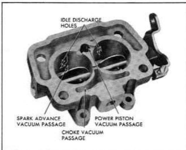
Fig. 6B-38 Passage Identification—Throttle Body
