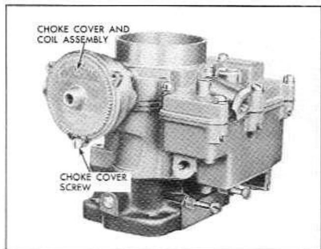
Fig. 6B-50 Choke Cover Assembly
