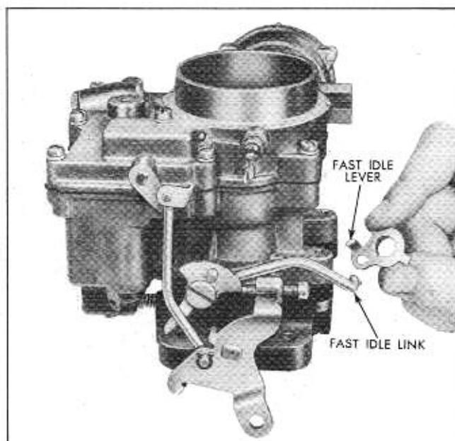
Fig. 6B-52 Removing or Replacing Fast Idle Lever
