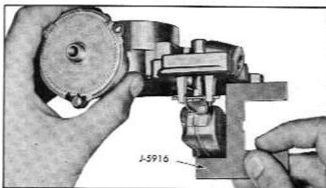
Fig. 6B-70 Checking Float Drop
