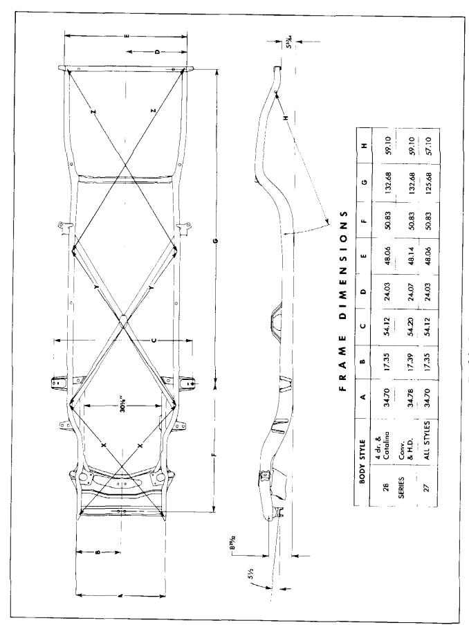
Fig. 2-1 Frame Checking Chart
