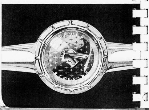
To distinguish models equipped with this device, the name "Power Steering" is added to the horn button of the 870 and Star Chief model's steering wheels. As illustrated, the name is in gold letters above and below the Indian head emblem. This identification will inform all drivers of the car that it is equipped with power steering, and to watch for the pleasures of driving this almost effortless way.
