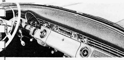
Available factory-installed or dealer-installed, this safety cushion provides a shock-absorbing surface through the use of fiber glass molded to fit the contour of the instrument panel. It is then trimly covered with durable Morrokide in a range of colors that harmonize with the instrument panel. It not only increases driving safety, but also cuts down reflected sun glare. Not available in cars with air conditioning.
