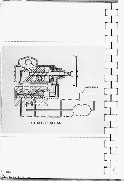
worm and ball nut, power piston and rack, and the power cylinder are all in-line. Since the valve is mounted on the top side of the gear housing, external oil passages between the valve and the cylinders are no longer necessary. Therefore, all external lines and hoses, except the pressure and return hoses between the pump and the valve, are eliminated and possibility of oil leakage due to line breakage is minimized.
