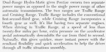
Cruising Range offers the ideal power for highway driving or cruising on the boulevard. The moment the fourth gear is reached, Pontiac's Economizer Rear Axle – with very low ratio of 3.08 or 3.23—allows the engine to work easily and effortlessly with substantial power and maneuverability. Worthwhile gasoline savings should result. The motor is quieted—makes for more restful, relaxed highway driving.
