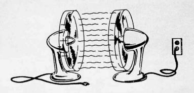
the blades. This circulating oil rotates the other "torus" member, which in turn drives the transmission. Because engine power is transmitted this way through a liquid, it is called fluid coupling.
