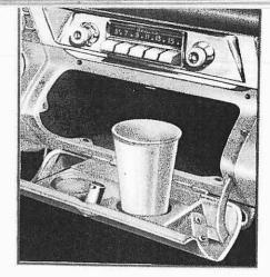
The relocation and new design of the glove compartment, first introduced in 1955, has been retained for 1956. It is easily accessible to both driver and front-seat passengers and has proven to be one of Pontiac's most popular interior features. But, in addition to this change, Pontiac also placed two depressions on the back of the glove compartment door for beverage containers. Thus, you have a handy place to put beverage containers when you frequent drive-in restaurants or make long trips.
