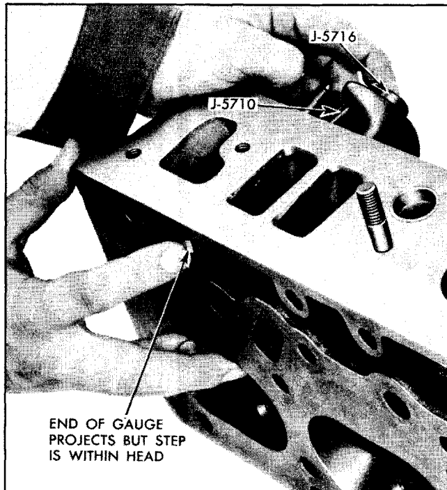
Fig. 6-40 Checking Length of Valve Stem
