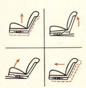
FRONT LEVER—By pulling up on this lever and pushing your body back, you can raise the front of the seat to any one of six positions. Pushing down gives you the reverse action. REAR LEVER—When you pull up on this lever and lean your body forward, the back of the seat will rise to any one of six positions. Pushing down gives you the reverse action. CENTER CONTROL—Regulates ten-position, forward-and-aft seat travel.
