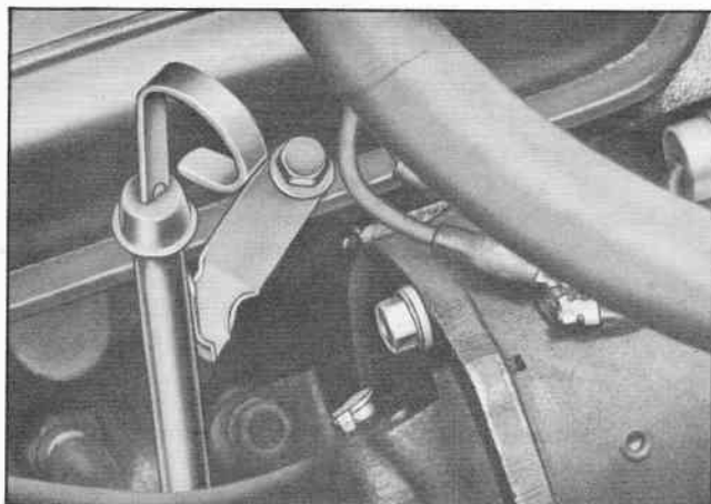
Fig. 5 Dip Stick Installed
