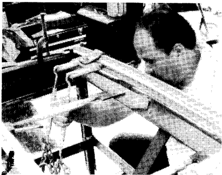
Steel plates attach to the top bar of the frame. Then Jerry attaches turnbuckles and tightens them to remove the twist in the top bar. He uses a gauge to determine when it's back to original straightness.
