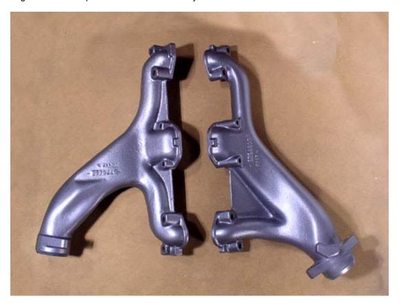
Alternative schemes that work with V8s into early chassis are OTC headers or custom headers. The 3-tube headers will fit in really tight places, like a 1979 Grand Prix. 4-tube headers require more room, but the 1<sup>st</sup> generation Firebird headers are easily modified to work...
