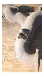
This adaptor was used for all dual exhaust cars from 56 to 58. I believe this elbow is sold as an after market item by Ames or CPR. I do not use the adaptor on my car; the custom exhaust pipe has the bend in it that allows it to be bolted directly to the manifold.
