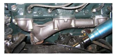
57 and 58 driver's side manifolds are the same. Note how the manifold exits to the front to clear the steering box. This is the adaptor Rick mentioned that directs exhaust to the rear.
