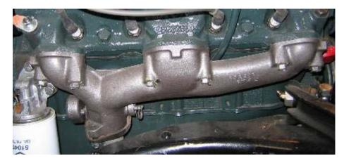
1957 through 1960 passenger side exhaust manifolds are interchangeable.
