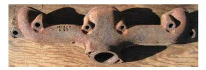
This manifold will work fine on the 57 engine. But with this manifold installed on the engine, the engine would not fit in 55 through 58 cars because the manifold would hit the steering box. If you decide to use stock Pontiac exhaust manifolds (probably the most cost effective option), you need to check what kind of clearance you have and select the appropriate manifold.
