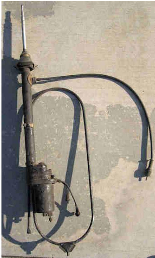
Power Antenna – Type I 1955 All Models 1956 Station Wagons Only Mast Lead Aluminum Storage Tube Upper End of storage tube clamps to antenna mast tube Crimped end of storage tube with drain at bottom loop of tube Short power leads with rubber boots
