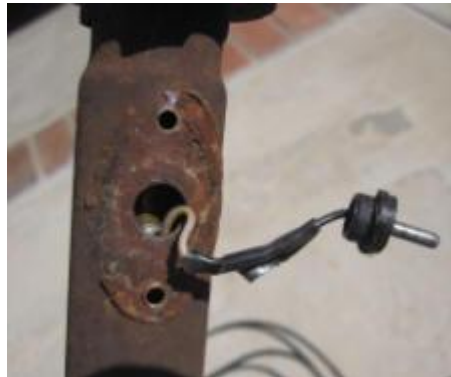
Pin and grommet spliced to new mast lead
