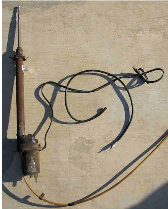
Power Antenna –Type II 1956 All models except Station Wagon Mast Lead Nylon Storage Tube Storage Tube clips to fuel tank flange Felt filter in drainage end of tube Long siamese power lead, no boots
