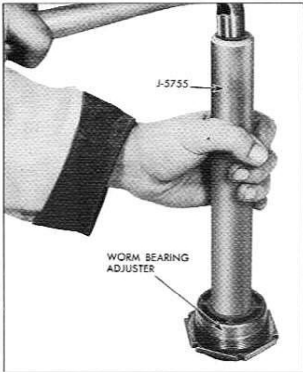
Fig. 9-15 Replacing Bearing Cup in Worm Bearing Adjuster
