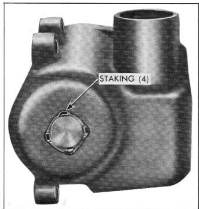
Fig. 9-45 Housing End Plug Staked
