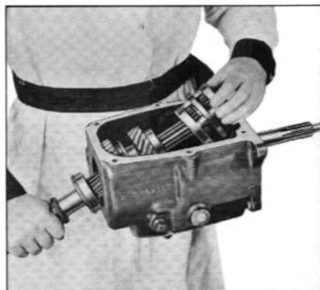
Fig. 7-18 Removing Synchronizer from Main Shaft
