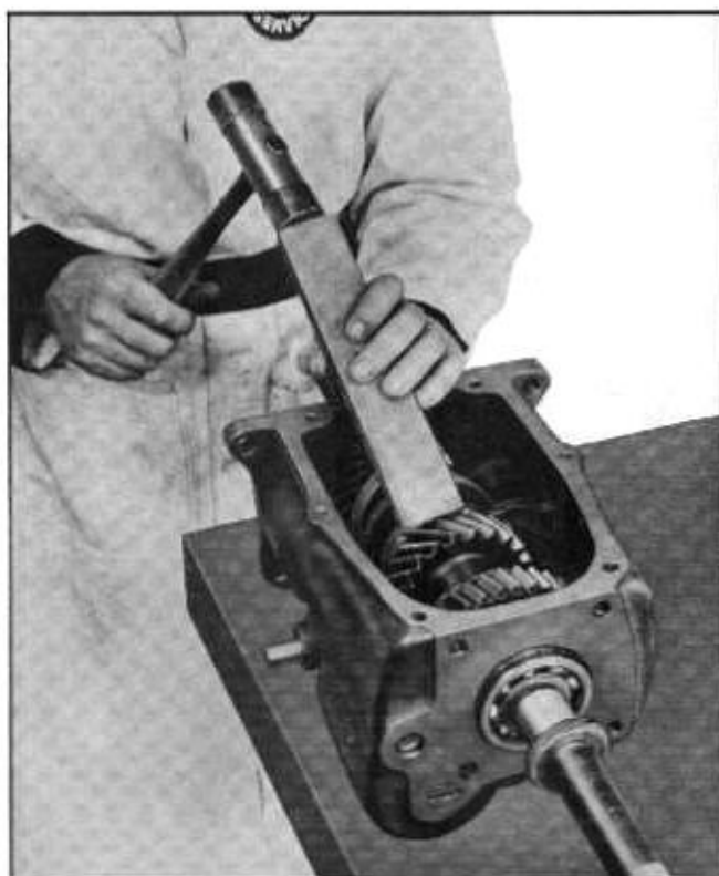
Fig. 7-17 Freeing Transmission Rear Bearing from Case
