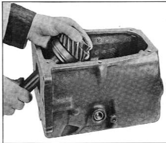
Fig. 7-23 Removing Main Drive Gear
