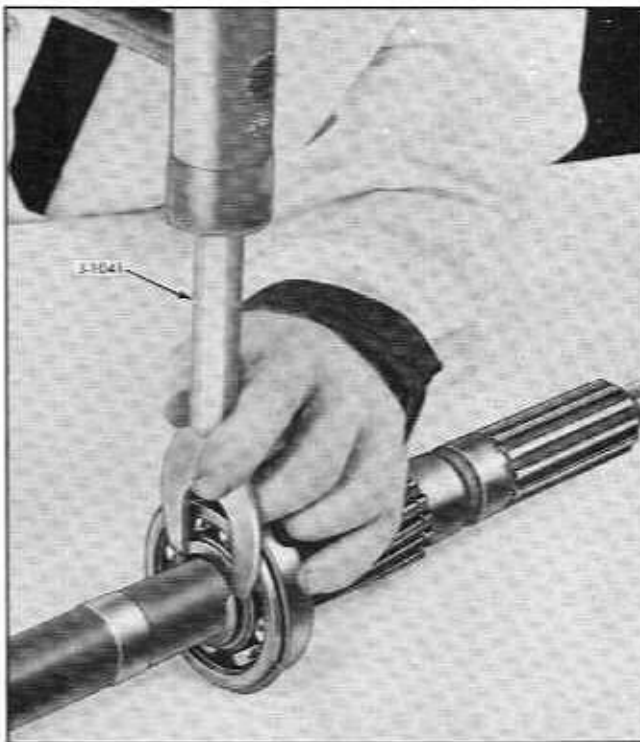
Fig. 7-28 Removing Rear Bearing Snap Ring
