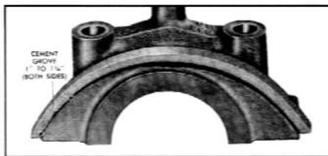
Fig. 6-31 Rear Oil Pan Gasket Positioned in Bearing Cap
