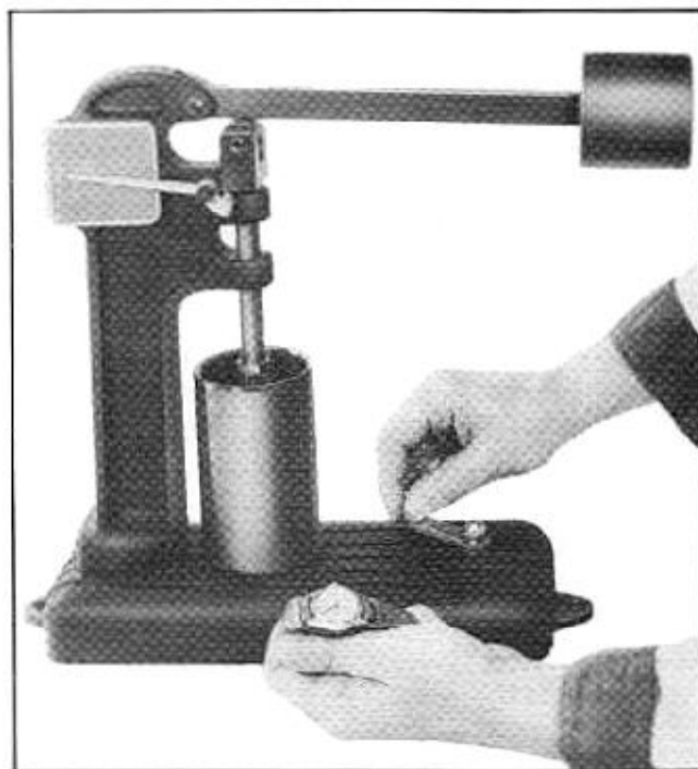
Fig. 6-53 Testing Leakdown Rate
