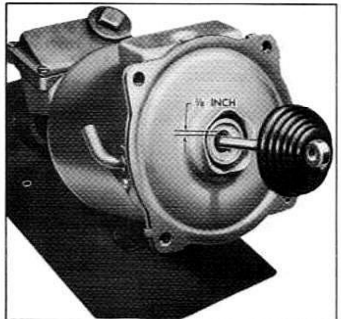
Fig. 5-34 Clearance Between Push Rod and Plunger
