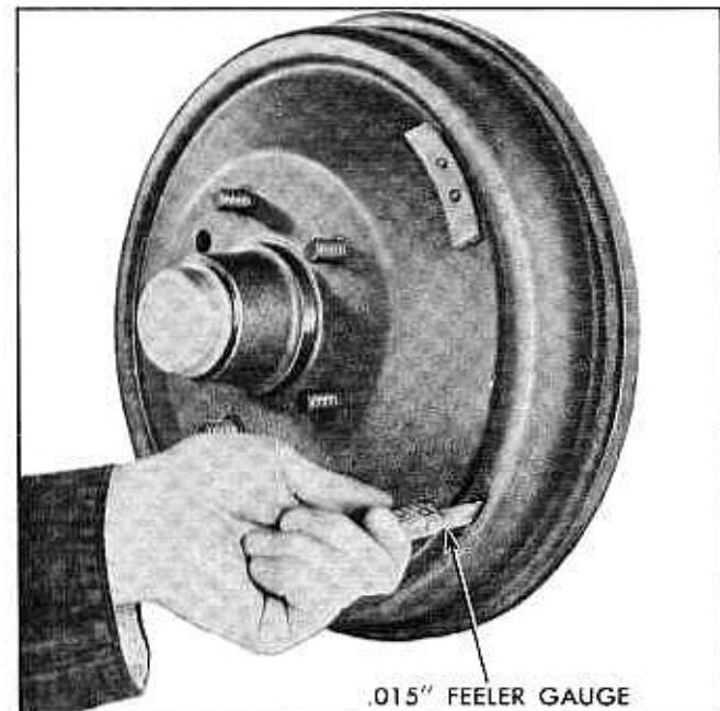
Fig. 5-9 Checking Lining to Drum Clearance
