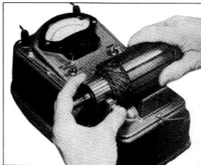
Fig. 12-16 Bar-to-Bar Test for Open Armature
