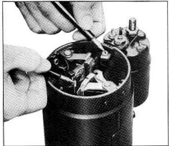
Fig. 12-30 Testing Field Coils for Open Circuit
