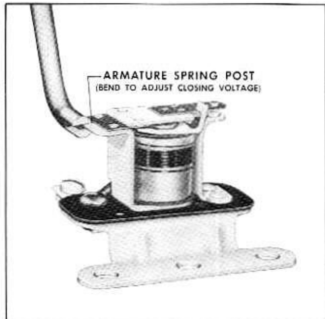
Fig. 12-71 Adjusting Relay Closing Voltage
