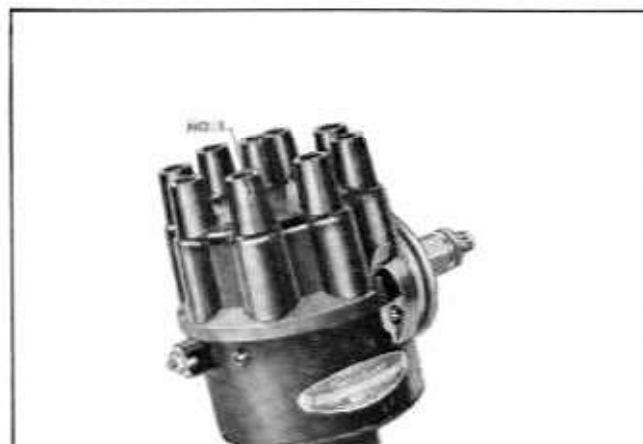
Fig. 12-55 Location of No. 1 Spark Plug Cable Terminal
