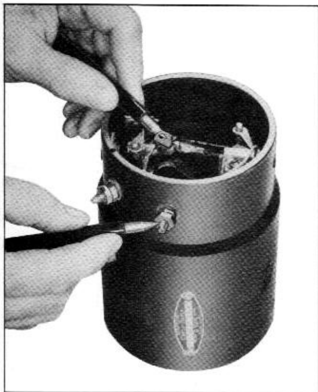
Fig. 12-18 Testing Field Coils for Open Circuit
