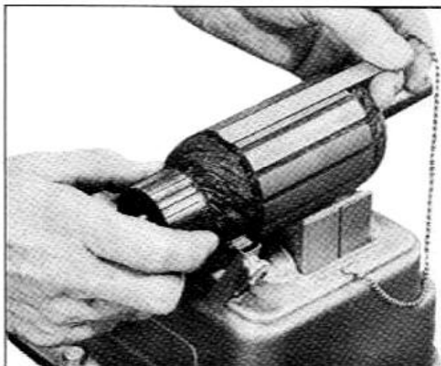
Fig. 12-15 Testing Armature for Shorts
