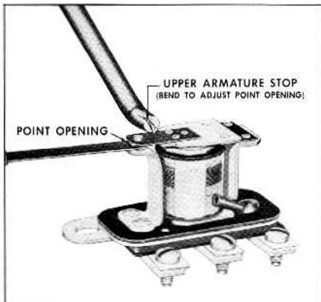
Fig. 12-70 Adjusting Contact Point Opening
