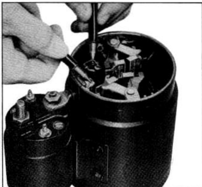
Fig. 12-32 Testing Shunt Coil for Open Circuit
