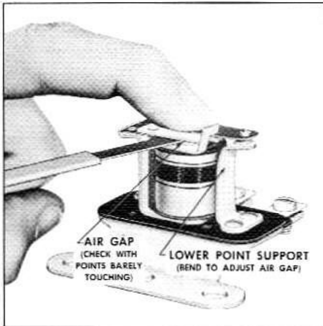
Fig. 12-69 Adjusting Air Gap
