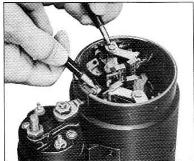
Fig. 12-31 Testing Field Coils for Ground
