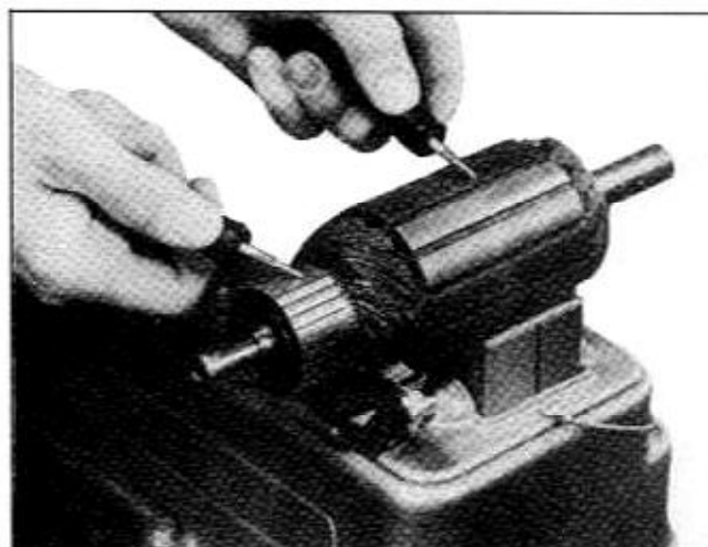
Fig. 12-17 Testing Armature for Ground
