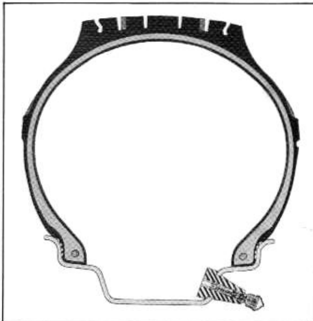
Fig. 10-1 Cross Section of Typical Tubeless Tire
