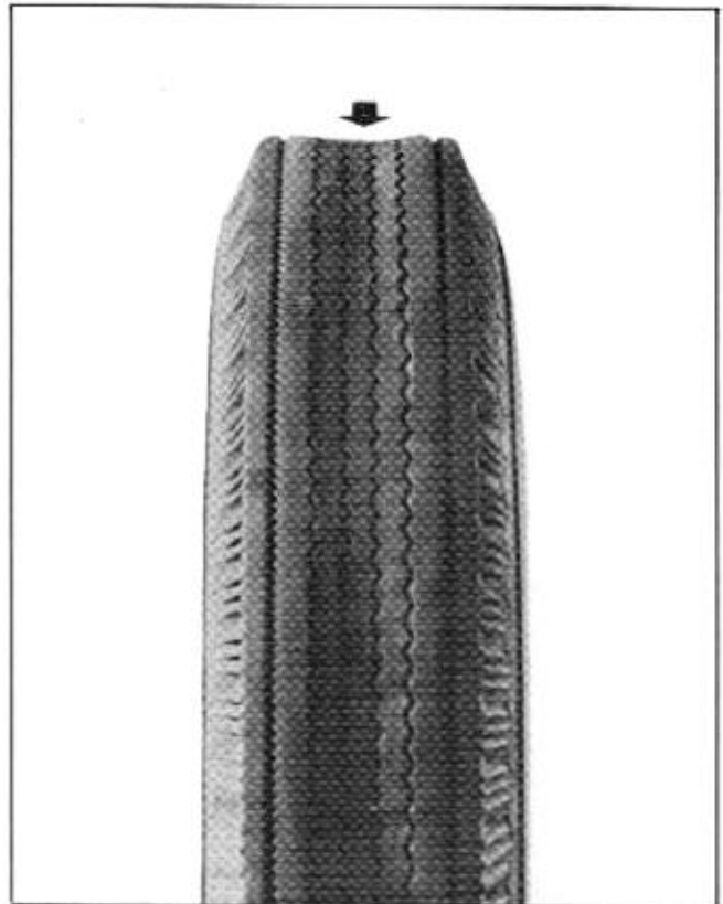
Fig. 10-4 Wear from Overinflation
