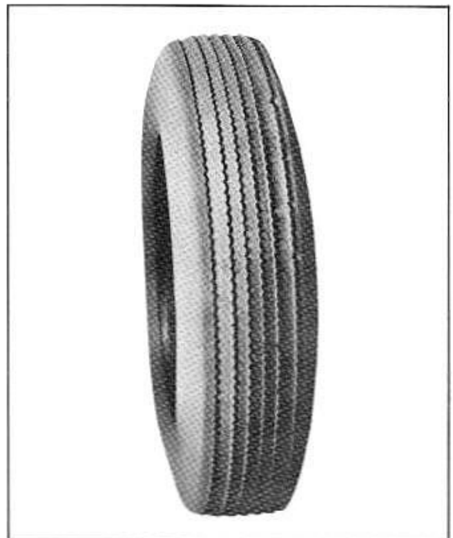
Fig. 10-6 Toe-in or Toe-out Misalignment Wear
