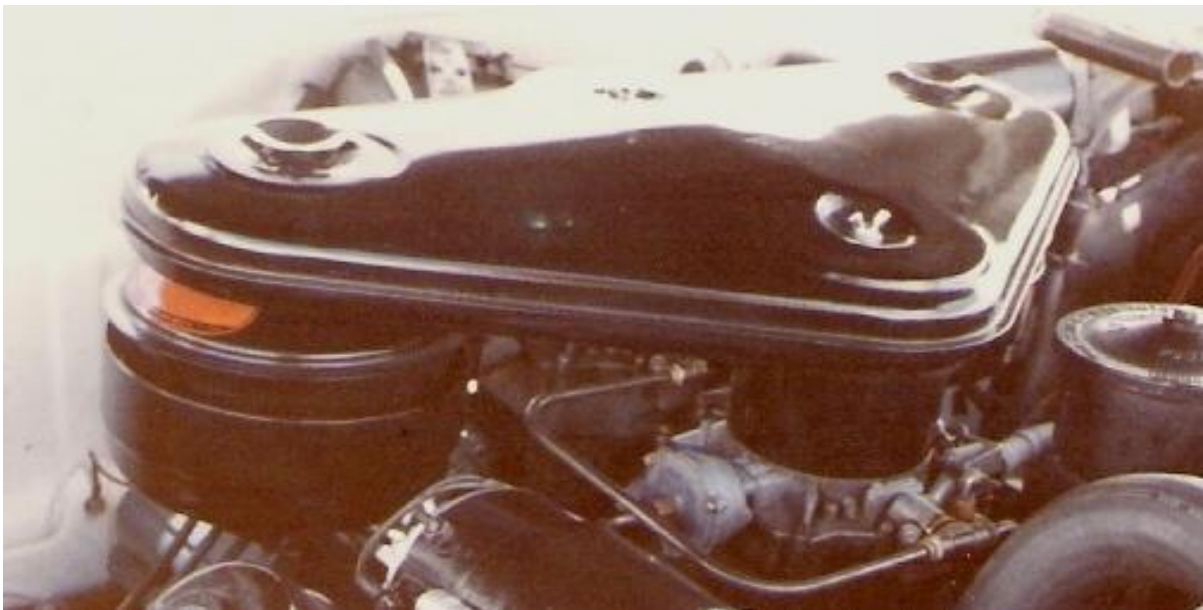
'56 Caddy batwing modified for '56 Pontiac (c.1979) (Photo credit: Len Sokol)
