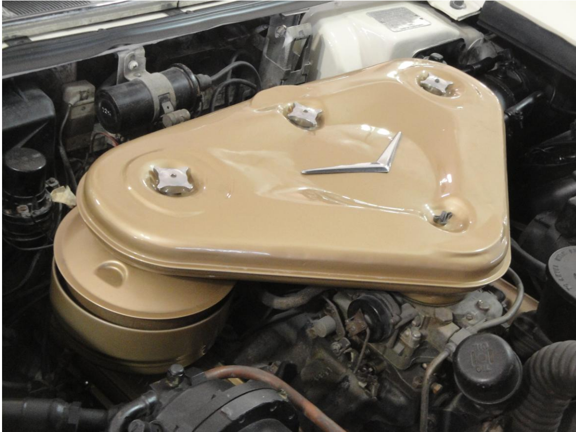
'57 Eldorado Brougham batwing (Photo credit: Len Sokol) Notice large recessed area in center. This was needed due to lowered body and hood on only the Brougham models. Unique and extremely low in production quantity.
