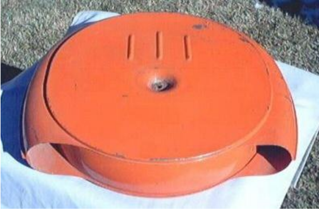
Air cleaner used on mid-50's Buick, Olds, Caddy
