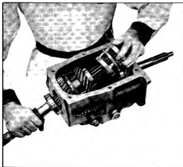
Fig. 7-13 Removing Synchronizer from Main Shaft
