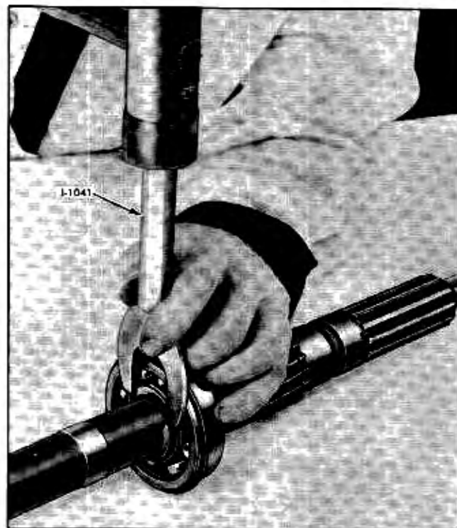
Fig. 7-23 Removing Rear Bearing Snap Ring
