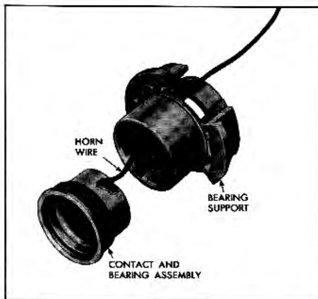
Fig. 7-10 Contact and Bearing Support Assembly
