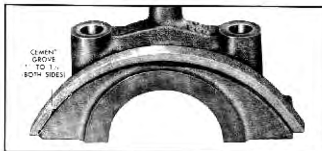
Fig. 6-30 Rear Oil Pan Gasket Positioned in Bearing Cap
