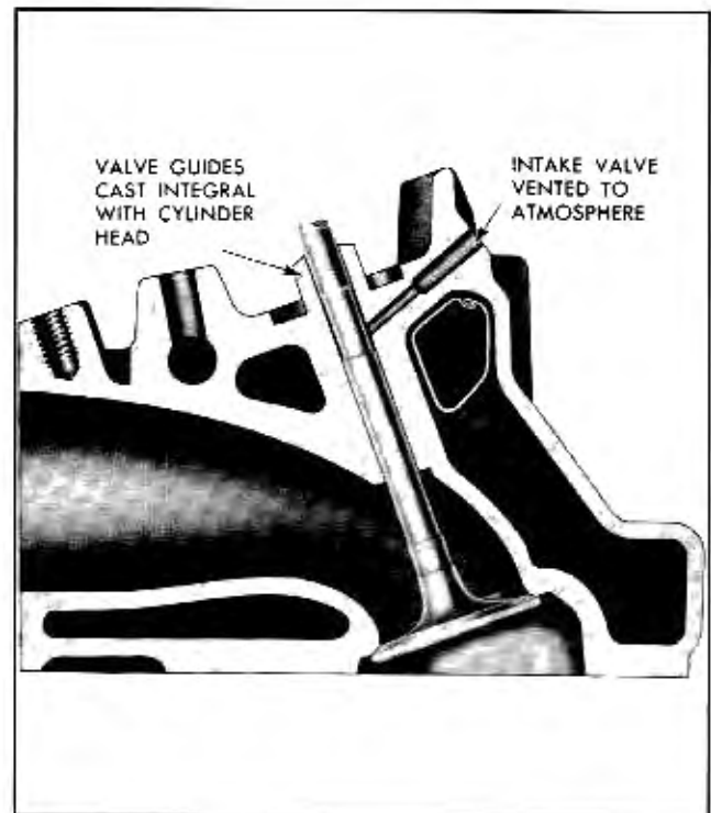
Fig. 6-8 Cross Section View of Intake Valve Guide Vented to Atmosphere
