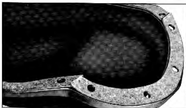
Fig. 6-31 Front Oil Pan Gaskets Overlapping Side Gaskets
