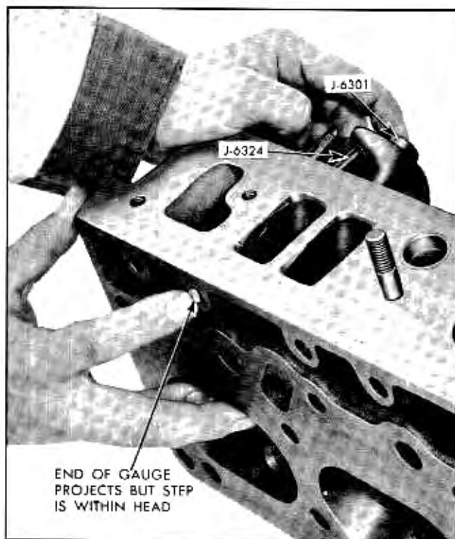
Fig. 6-44 Checking Length of Valve Stem
