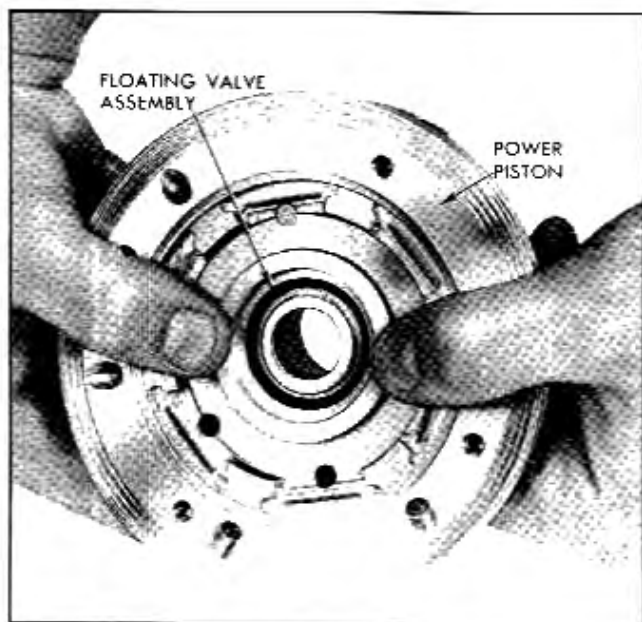
Fig. 5-67 Replacing Floating Control Valve
