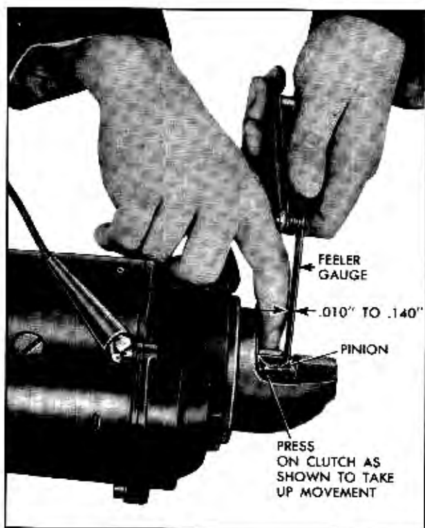
Fig. 12-43 Measuring Pinion Clearance
