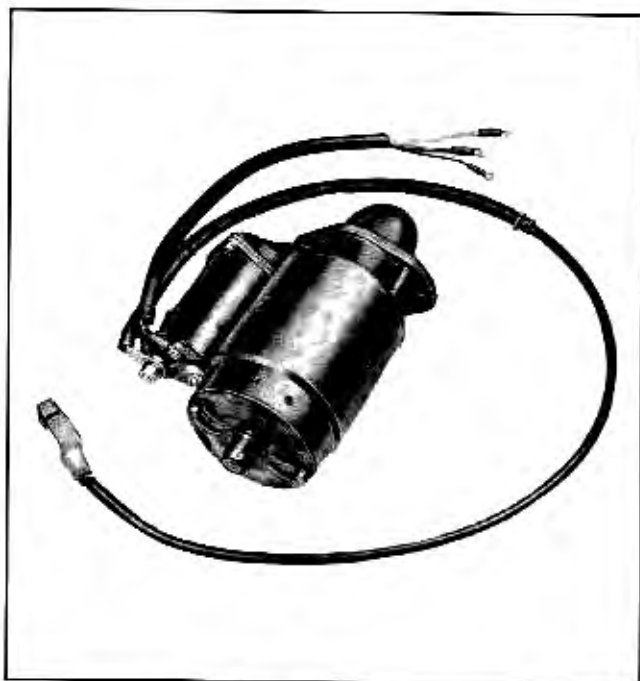
Fig. 12-44 Wires and Cable Connected to Solenoid
