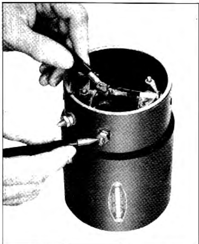
Fig. 12-23 Testing Field Coils for Open Circuit
