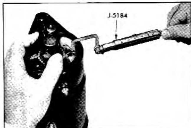
Fig. 12-18 Checking Brush Spring Tension
