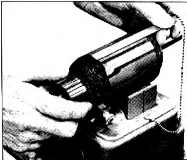
Fig. 12-20 Testing Armature for Shorts
