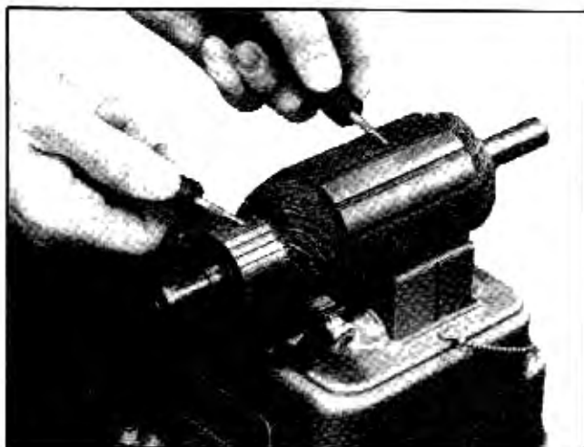
Fig. 12-22 Testing Armature for Ground
