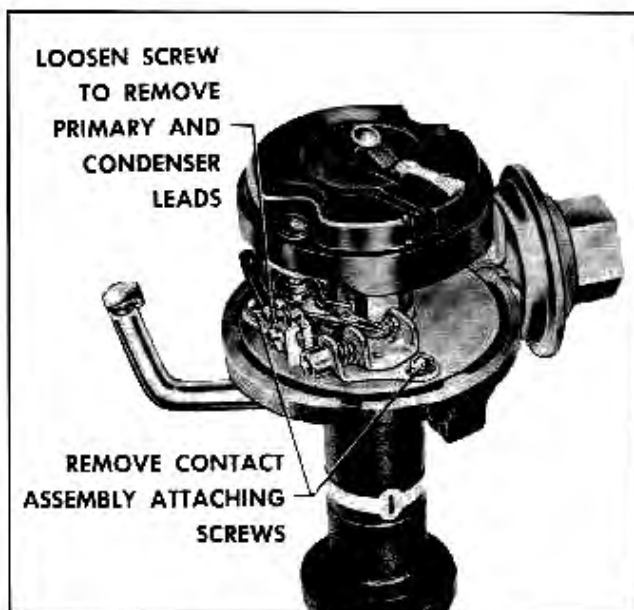
Fig. 12-55 Distributor Contact Details
