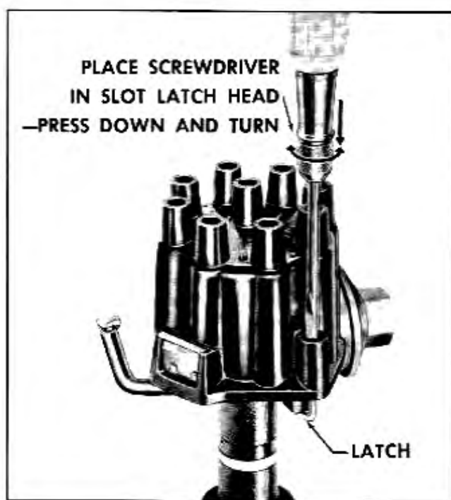
Fig. 12-54 Removing Distributor Cap
