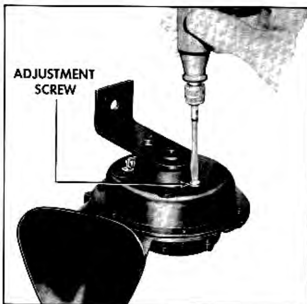
Fig. 12-72 Adjusting Current Draw of Horn
