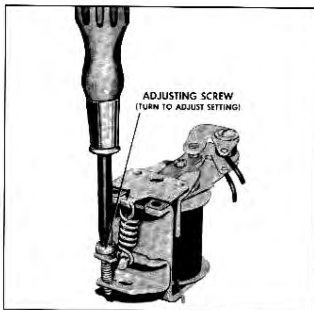
Fig. 12-16 Adjusting Voltage Regulator Setting (Lower Contacts)
