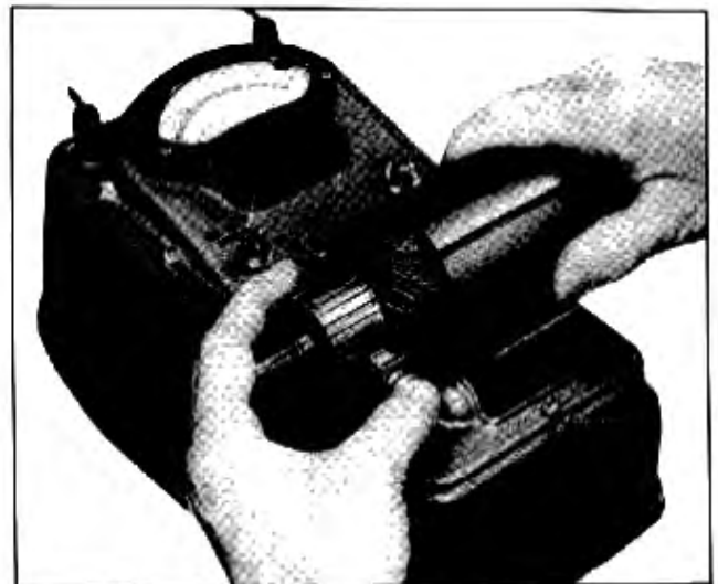
Fig. 12-21 Bar-to-Bar Test for Open Armature
