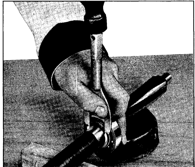
Fig. 7-29 Removing Rear Bearing Rear Snap Ring with Tool J-1041
