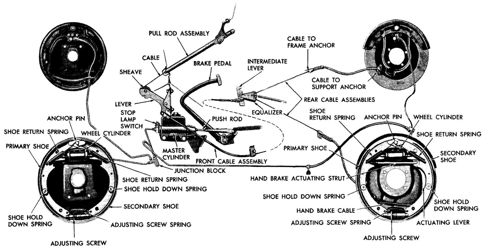
Fig. 5-1 Diagram of Complete Brake System
