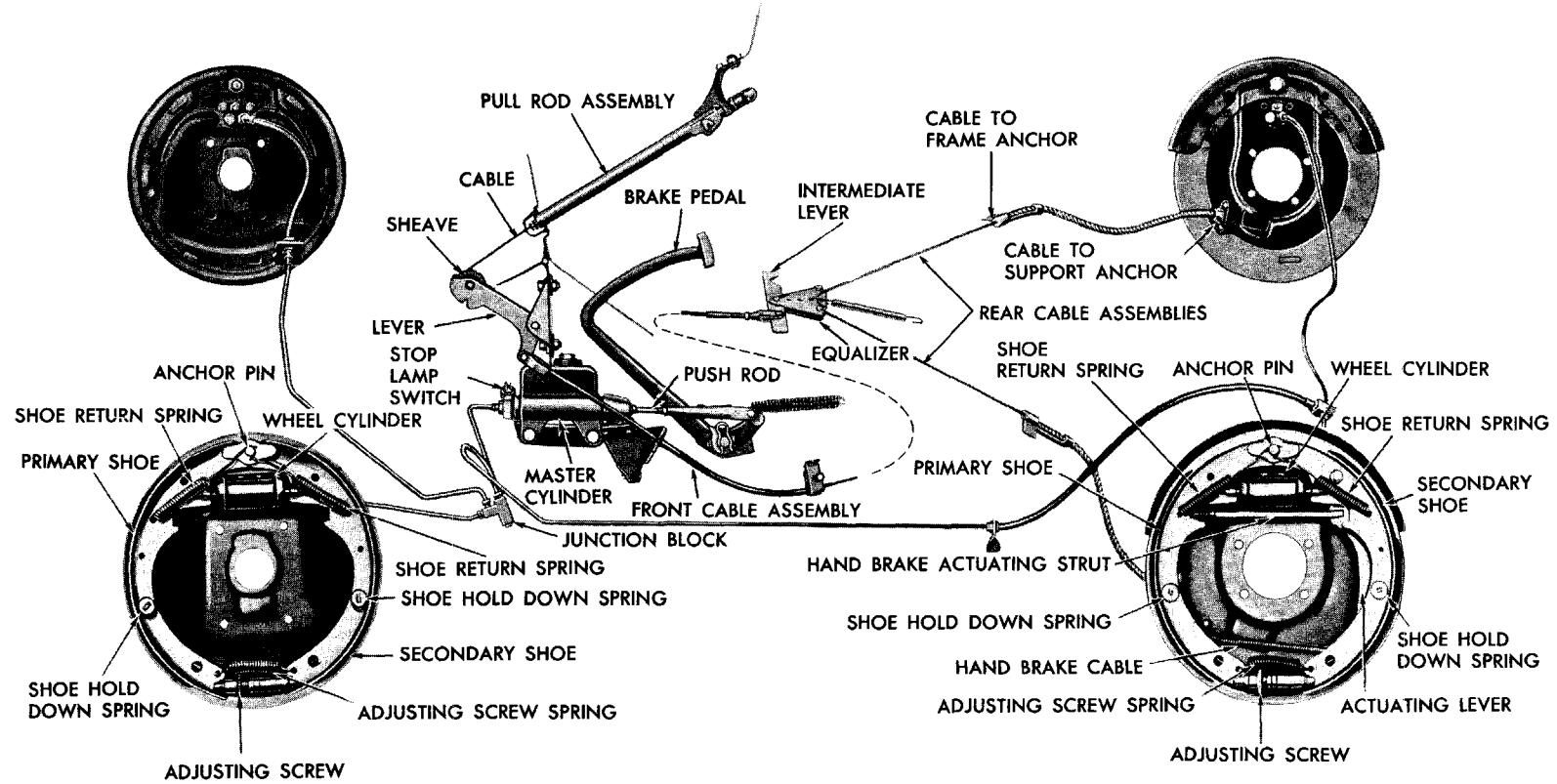
Fig. 5-1 Diagram of Complete Brake System
