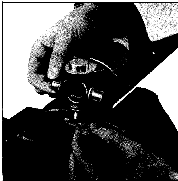
Fig. 4-53 Placing Washers Inside Bearing of Fixed Yoke Member
