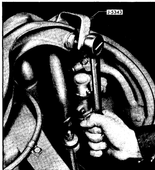
Fig. 3-10 Adjusting Caster or Camber
